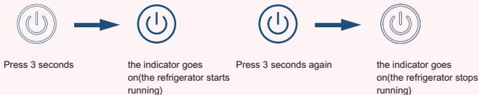
Press 3 second--the indicator goes on (the refrigerator starts running)--press 3 seconds again --the indicator goes off(the refrigerator stops running)
