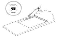
Seal the cut edge of the worktop using silicone sealant or PVA adhesive.
