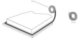
Stretch out and stick the supplied tape along the underside edge of the hob, ensuring the ends overlap. Trim off any excess tape and dispose of it.
