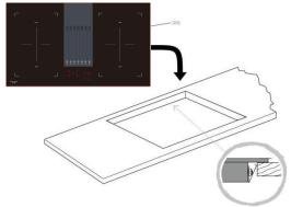
Once the worktop edge has cured, and the tape is fitted, position the hob into the cutout in the worktop. Apply gentle downwards pressure onto the hob to push it into the worktop ensuring a good seal around the outer edge.
